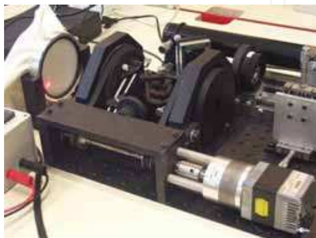
Fig. 18. Photograph of the mechanical device of the rotating texturometer used in the extensometry application.
