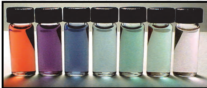
Fig. 24. The effect of size quantization: light emission from gold colloids with varying size of nanoparticles, smallest particles emit violet and the largest emit red color.
