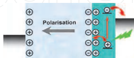
Fig. 10. A schematic display of an anode/ blocking layer / active layer/ cathode photosensor.
