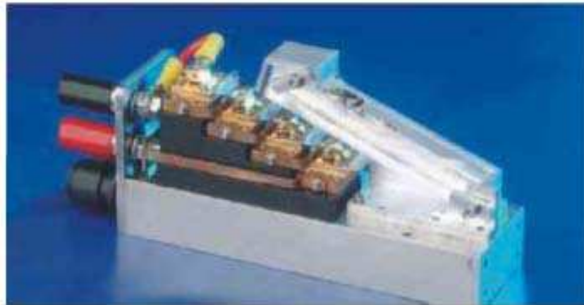
Fig. 22. The integrated fiber-coupled output module from laser array laser arrays packaged by conduction heat sink.
