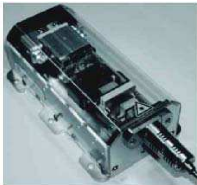
Fig. 21. The integrated fiber-coupled output module from laser array stacks packaged with micro-channel heat sink.
