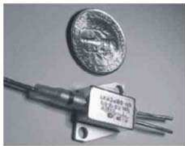
Fig. 18. The fiber-coupled output module from a single emitter.
