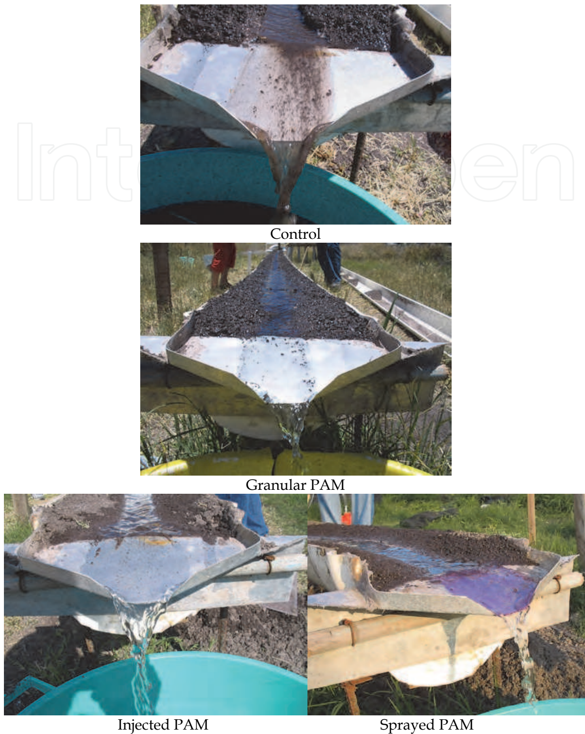
Fig. 5. Detachment in the furrows treatments with PAM and the control
