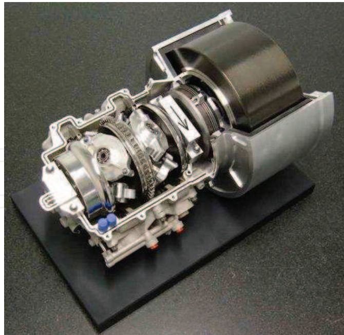
Fig. 2. Flywheel in a Kinetic Energy Recovery System (KERS) (courtesy of Flybrid Systems LLP, Silverstone, Northamptonshire, England)
