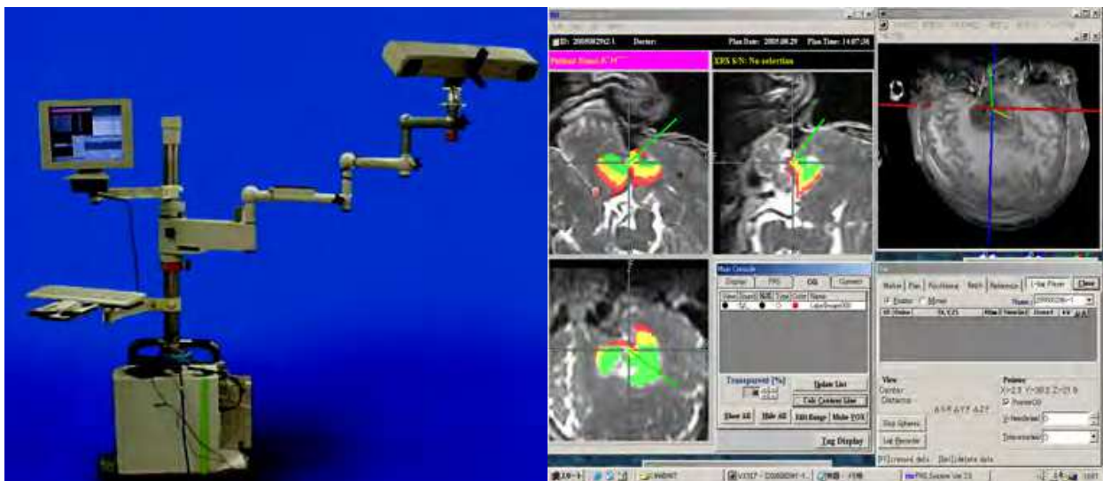
Fig. 5. Intraoperative neuronavigation system (PRS navigator; Toshiba Medical Co. Ltd., Tokyo, Japan) used in intelligent operating theater of TWMU ( left ) and its screen with color-coded safety areas of the tumor resection ( right ), showing areas located less than 5 mm, between 5 and 10 mm, and more than 10 mm to the pyramidal tract, which are demarcated, respectively, as red, yellow, and green.
