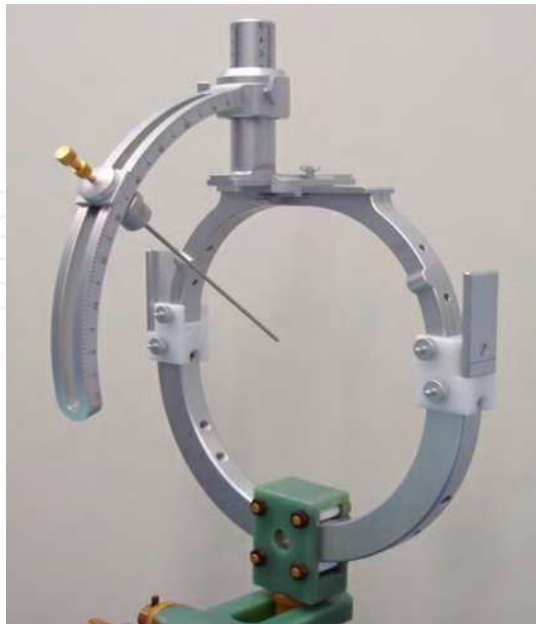
Fig. 3. Head-holder coil integrated with modified Komai stereotactic frame for stereotactically guided surgical procedures under the control of intraoperative MRI.
