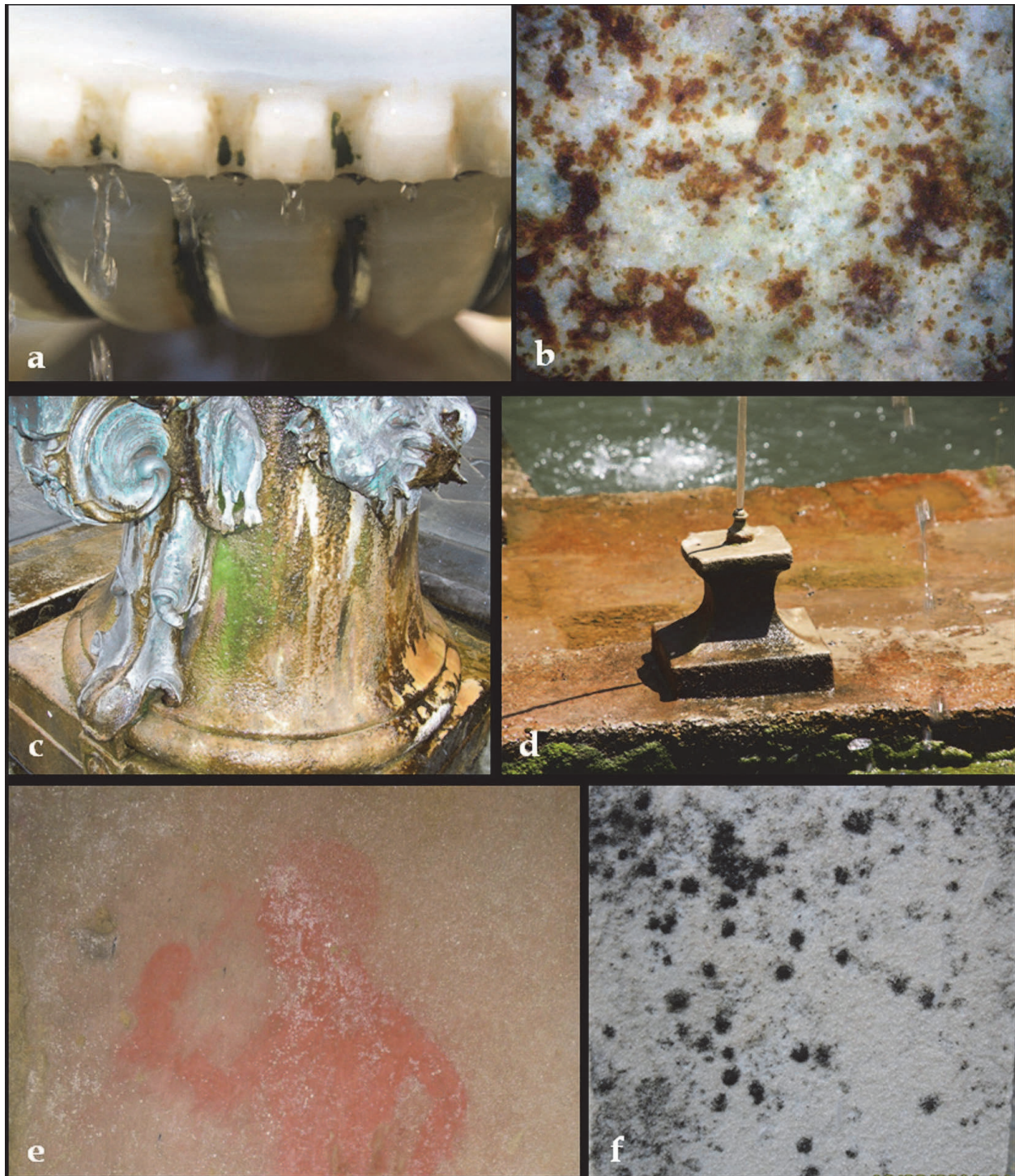
Fig. 6. Various typologies of biological colonization found on monumental stones: (a) green algae pustules and (d) microbial mat on artistic fountain from Alhambra complex, Granada (Spain); (b) diatoms brown pustules and (c) phototrophic biofilm developed on Tacca's fountains from Florence (Italy); (e) irregular whitish stains produced by actinomycetes in an Etruscan tomb from Chiusi (Italy); (f) microcolonial fungal growth on marble stone, from Trespiano monumental cemetery, Florence (Italy)
