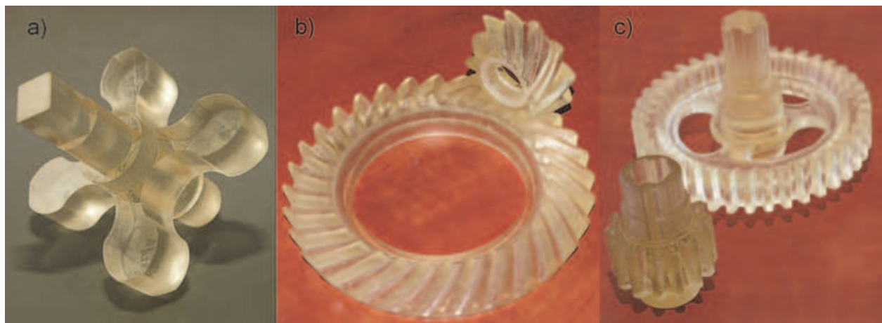
Fig. 4. Gear wheels made by SLA method: a) gear wheel of cycloidal profile, b) bevel gear wheels, c) cylindrical gear wheels
