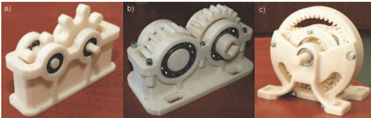
Fig. 5. Gears made by FDM method: a) single-stage gear with wheels of cycloidal profile, b) single-stage gear with wheels of involute profile, c) planetary gear
