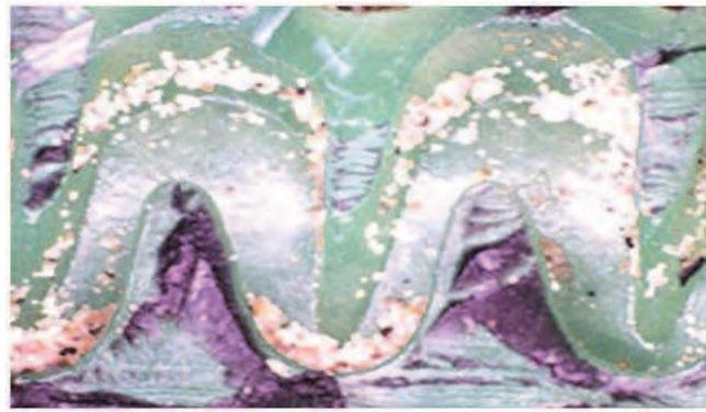
(a) starting stage of clogging
