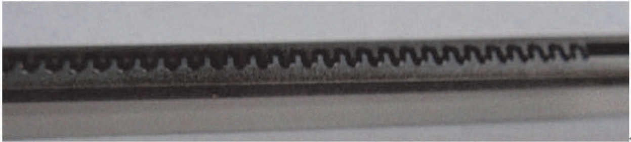
Fig. 34. Oblique teeth channel emitter obtained by assembling the wire-cutting samples and the RP sample
