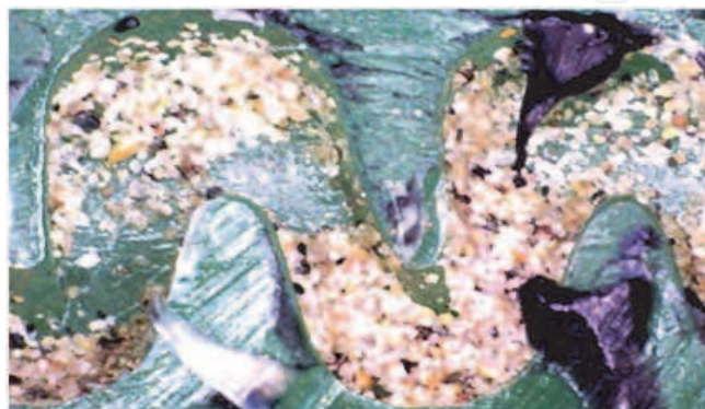
(b) developing stage of clogging
