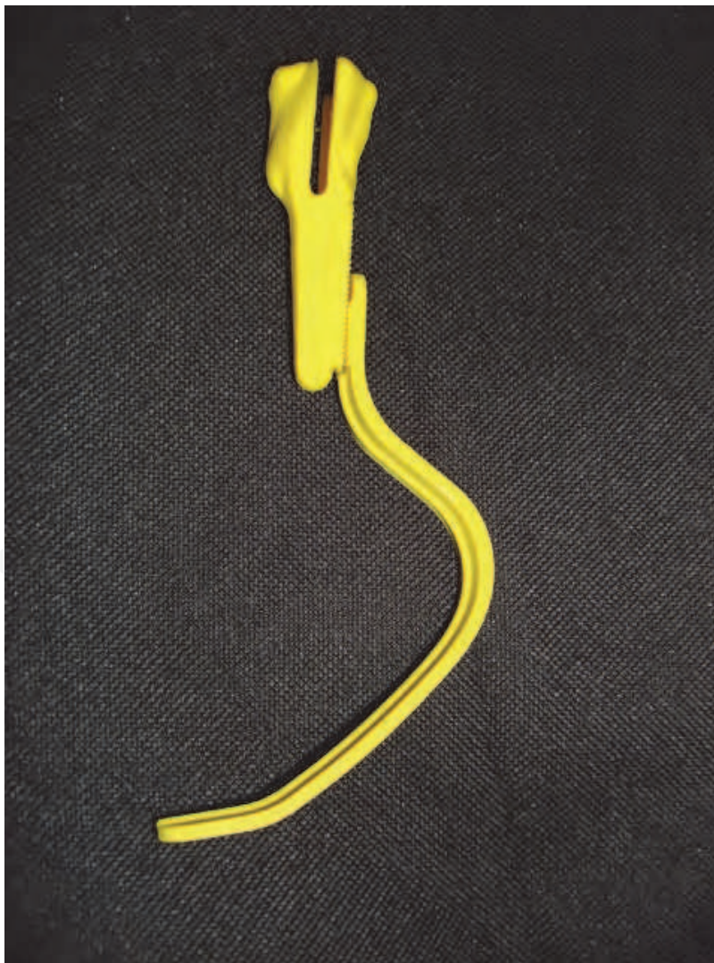
Fig. 15. Orthosis produced by means of the SLS rapid prototyping technique.
