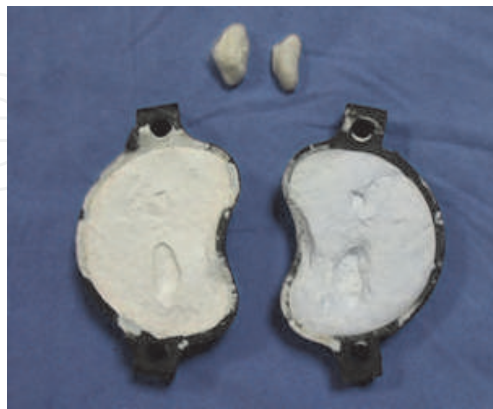
Fig. 4. Negative mould of the left mandibular condyle. gypsum fibrosum mould, open. Rapid prototyped PGA/PLA scaffolds in mandibular condyle bone defect reconstruction
