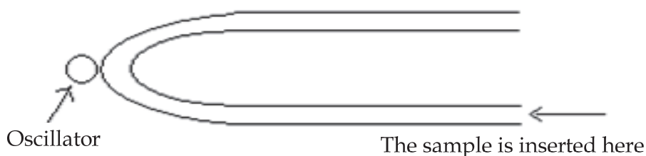
Fig. 7. U-shaped tube of digital density meter.
