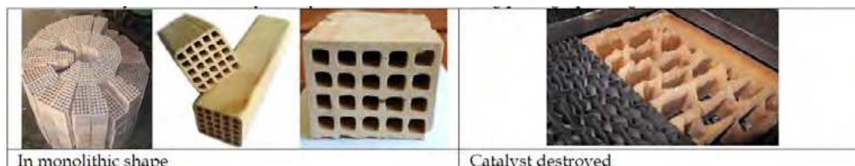
Fig. 14. View of a catalyst SCR.
