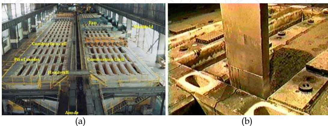
Fig. 1. a) Anode baking furnace building overview; b) Petroleum coke being unpacked from anode coverage by vacuum suction.
