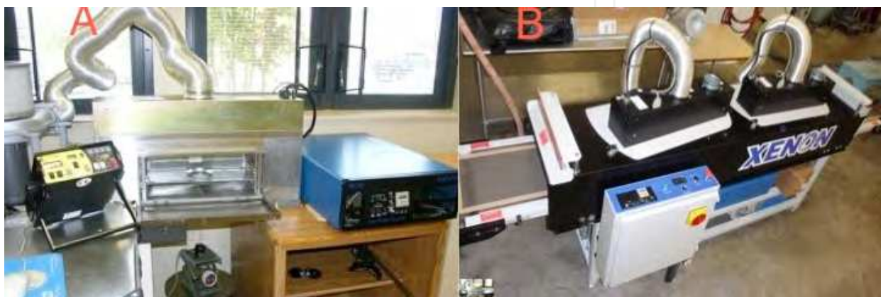
Fig. 3. A. SteriPulse XL-3000 batch PUV system; B. LHS40 continuous PUV system, as manufactured by Xenon Corporation (Wilmington, MA).
