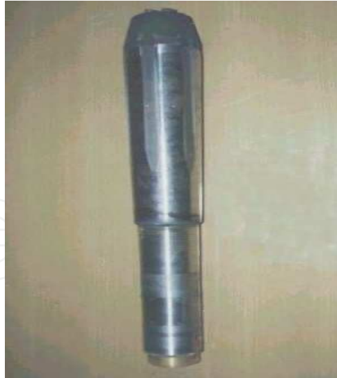
Fig. 7. Laboratory version of the flame jet pump system injection head (with permission of Professors Lazar and Sekula, Technical University of Košice, Slovak Republic)
