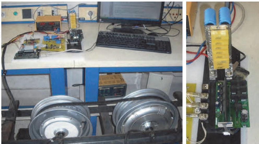
Fig. 8. Experimental setup for the in-wheel brushless motor drive validation and the IPM based power circuit.
