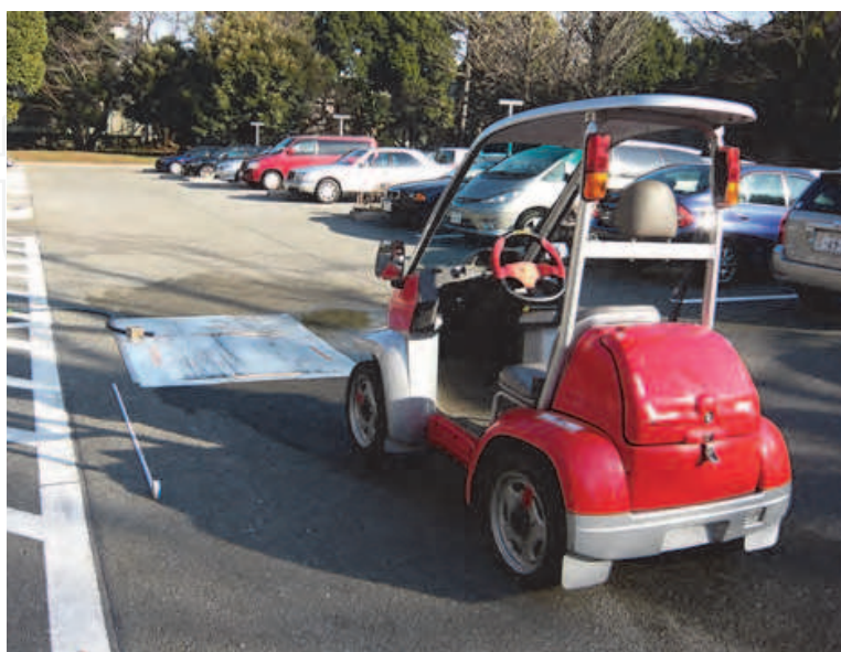
Fig. 11. Experimental electric vehicle and setting of slippery road for experiment.
