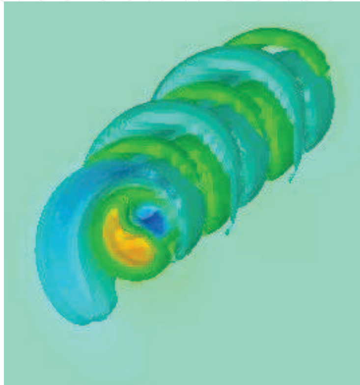
Fig. 7. Superposition upon the steady laminar basic state at Re = 3180 , U_0 = \frac{0.5}{\pi} , of its most amplified BiGlobal eigenmode at amplitude 0.1%. Axial spatial direction reconstructed using L_x = 2\pi/\beta , with \beta = 3.0 ; eigenvalue \omega_i = 0.04603 , \omega_r = 0.06072 González, Gómez-Blanco & Theofilis (2008).
