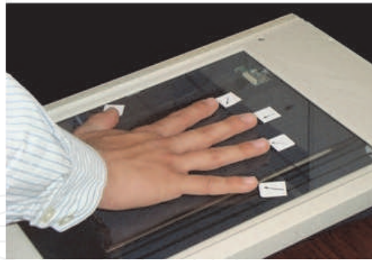
Fig. 4. Pegs on the scanner for hand positioning.
