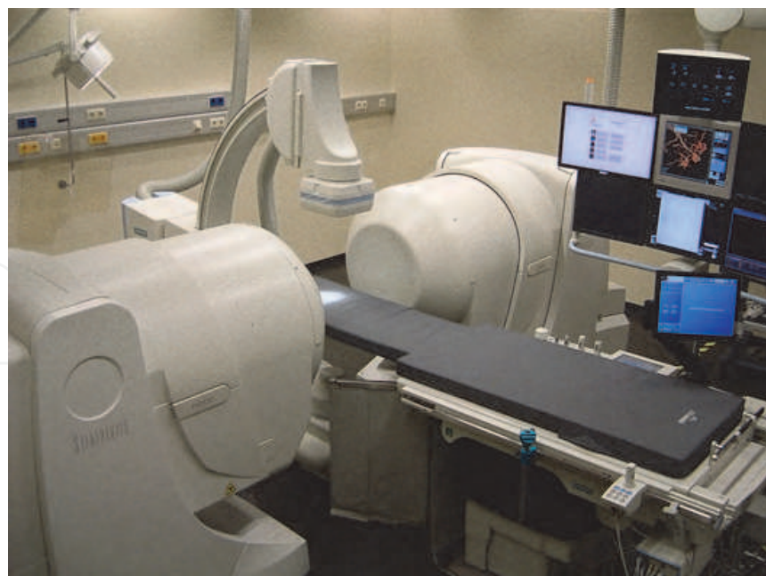
Fig. 3. Catheter suite with a magnetic navigation system (Niobe). Permanent magnets to both sides of the fluoroscopy table can be moved inside their casings to alter the magnetic field.
