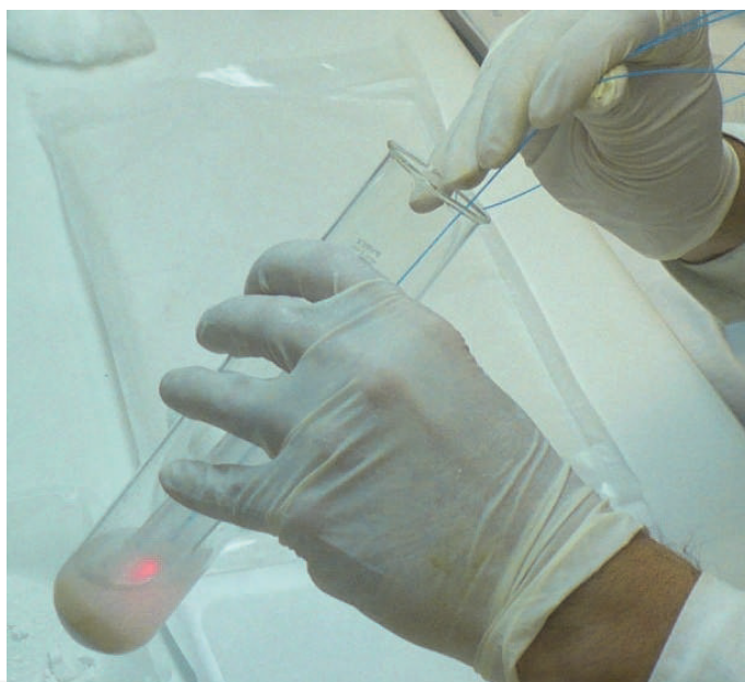
Fig. 1. Photograph of the special lucite test tube with copper mesh bottom (not seen) placed inside a standard glass laboratory test tube during in vitro fragmentation of an artificial infected kidney stone with a laser lithotripter.
