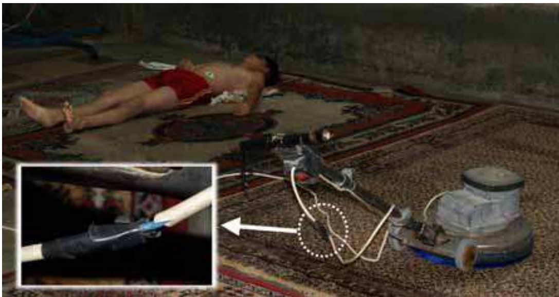
Fig. 22. A 17-year-old worker was dead due to electric shock in his workplace. The scene investigation revealed electrical leakage from the defect of the plastic sheath of the cable of carpet washing machine.
