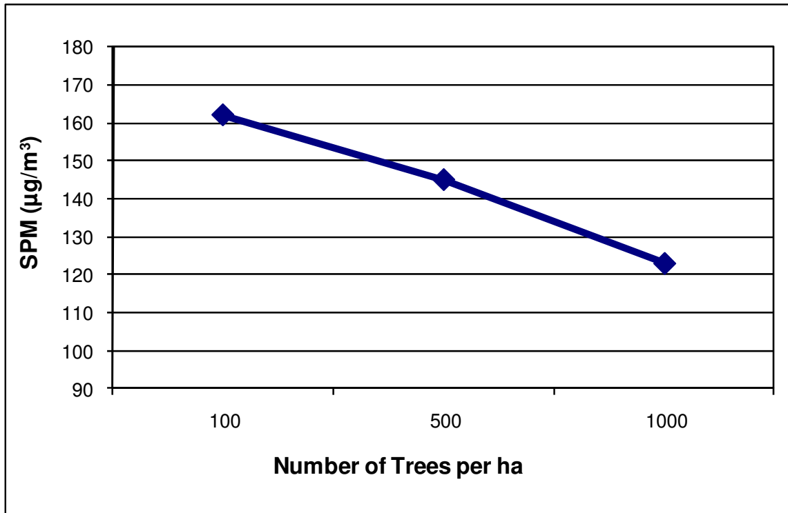
Fig. 2. Relationship between number of trees (per ha) and ambient SPM concentration (Slope: 0.04 and Intercept: 166.17)
