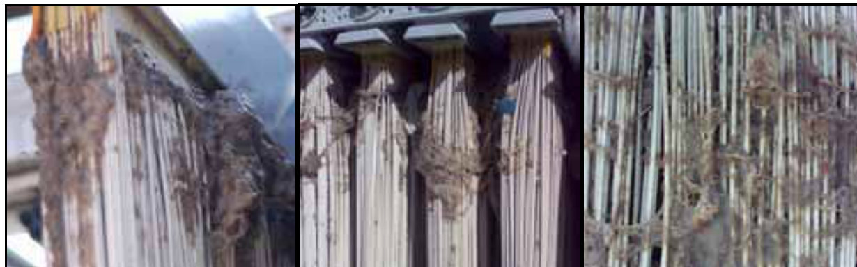
Fig. 2. a/b/c. Membrane module clogged. Debris can be observed located between the top headers modules forming a bridge between them (Morro Jable wastewater treatment plant, Canary Island, Spain; courtesy of CANARAGUA, S.A.)
