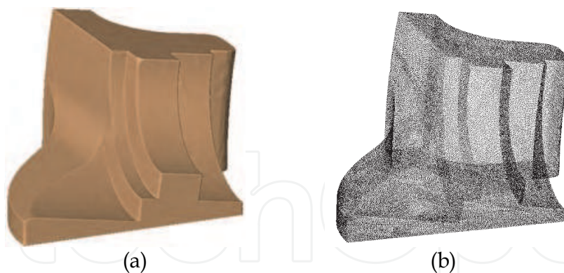
Fig. 9. Fan disk point clouds without noise. (a) Geometric model. (b) Original point clouds.
