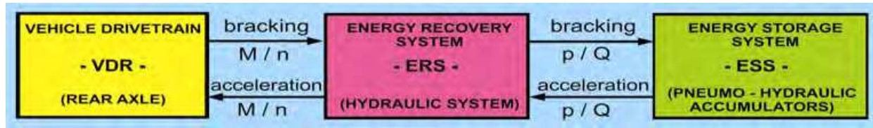
Fig. 3. Global systemic model of a motor vehicle equipped with a kinetic energy recovery system.
