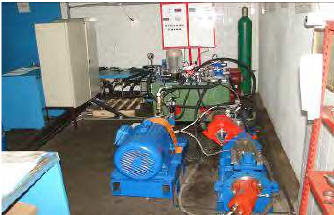
Fig. 24. Mechatronic stand for testing the kinetic energy recovery system – frontal view.
