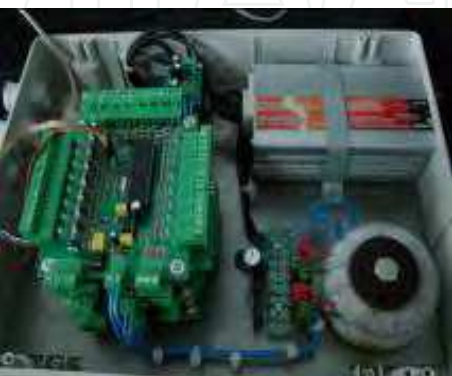
(g) Electronic drive and control subsystem
