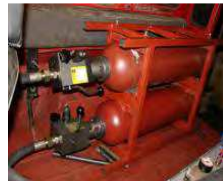
(e) The accumulators battery
