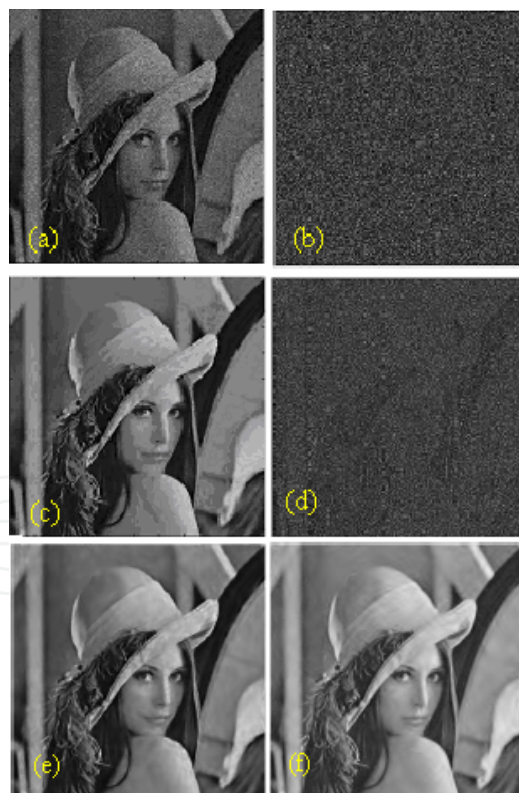
Fig. 17. A comparison of three despeckling methods acting in the wavelets domain; (a) noisy image (PSNR=21.4 dB), (b) speckle noise distributed following a Rayleigh law with unitary mean, (c) result obtained with the method based on 2D DT CWT (PSNR=31.4 dB), (d) 2D DT CWT method's noise, (e) result obtained with the method based on HWT (PSNR=32.5 dB), (f) result obtained with the method in [Argenti et al., 2006] (PSNR=31.1 dB).
