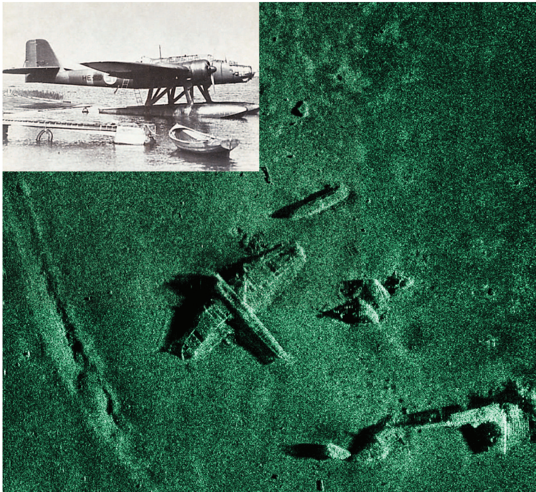
Fig. 18. SAS image of a German WWII Heinkel He 115 seaplane lying on the seafloor. Courtesy of the Royal Norwegian Navy. Photograph is from wikipedia.
