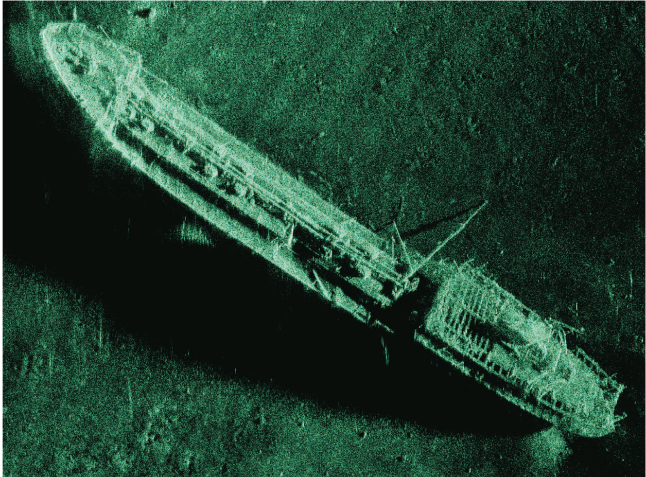
Fig. 16. SAS image of the wreck of the Norwegian tanker Holmengraa that was sunk during WWII in 1944. Courtesy of Kongsberg Maritime.
