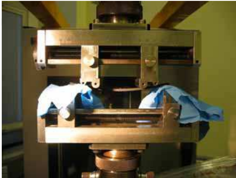
Fig. 10. Experimental setup for 4PBFT specimens
