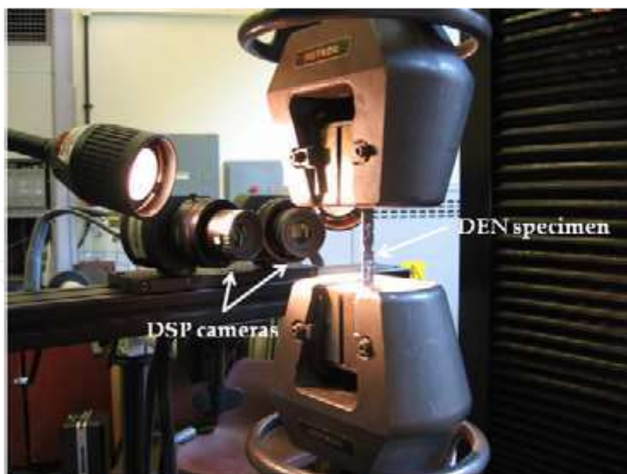
Fig. 9. Experimental setup for DEN specimens
