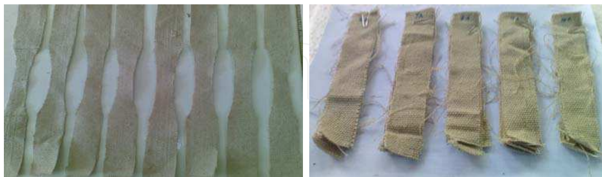
(a) Ramie woven for tensile testing
