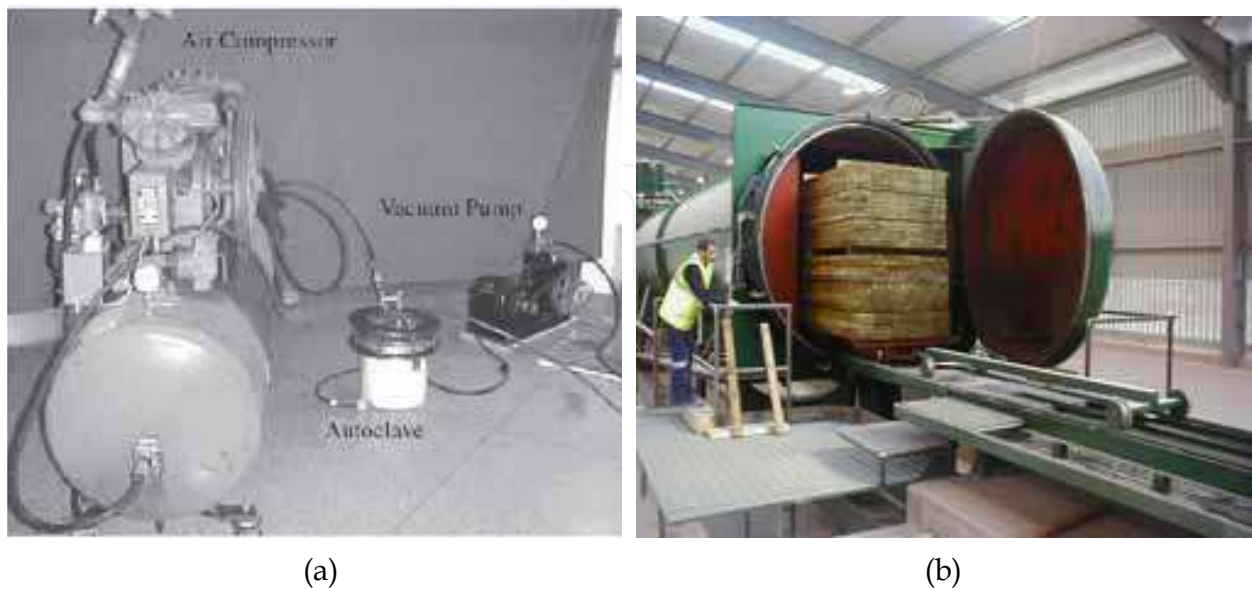
Fig. 25. Systems used to impregnate the wood (a) impregnating equipment in experimental use (b) impregnating equipment in plant use
