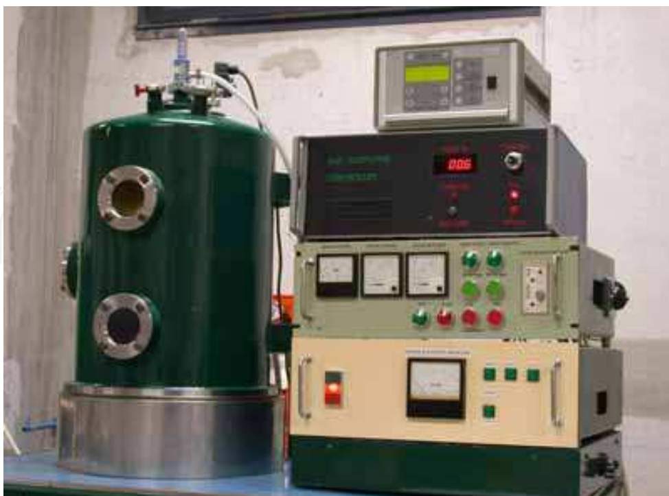
Fig. 3. The view of the system used for deposition of carbon coatings by PACVD method
