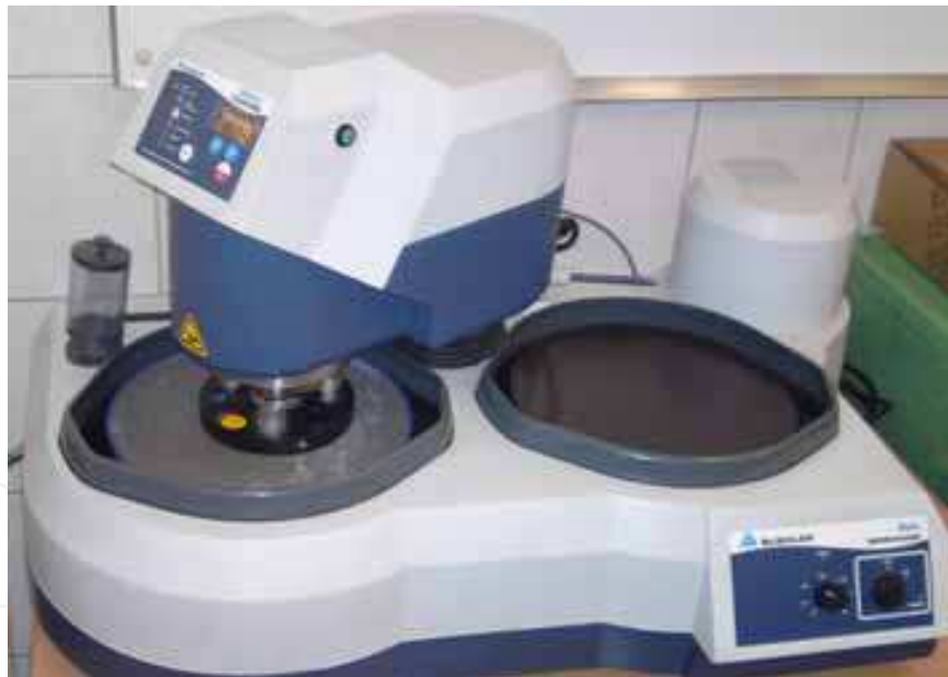
Fig. 4. The overall view of the Beta 2 dual platen grinder-polisher machine equipped with Vector power head and specimens holder
