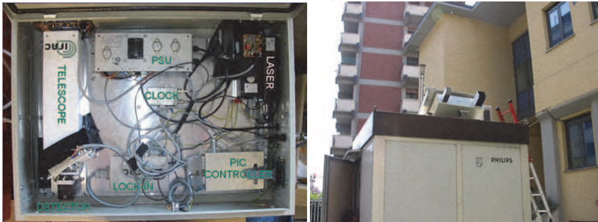
Fig. 12. The instrument opened (left) and installed on the roof of the ARPAT, PM-monitoring station in Florence (I) (right)
