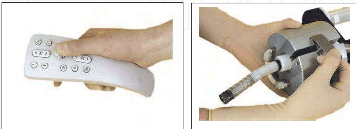
Fig. 8. Hand-Held device and the instrument tip in the driving unit.
