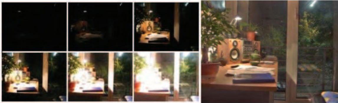
Fig. 5. An example of HDR creation from multiple differently-exposed images. (Source exposures by Grzegorz Krawczyk)
