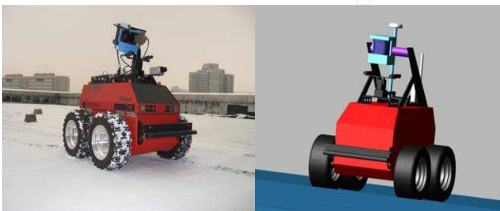
Fig. 10. ATRV2 and its model in ADAMS
