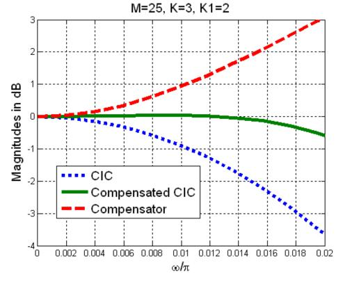
Fig. 5. Wideband CIC compensation using the Compensation method 1.
