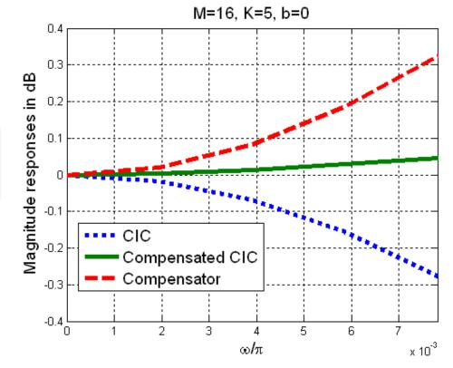
Fig. 3. Magnitude responses of CIC, Compensator and cascaded CIC-compensator.
