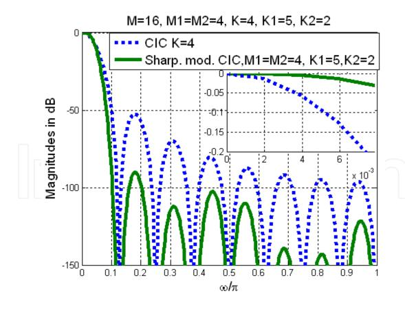
Fig. 12. Modified sharpening and CIC filters magnitude responses.
