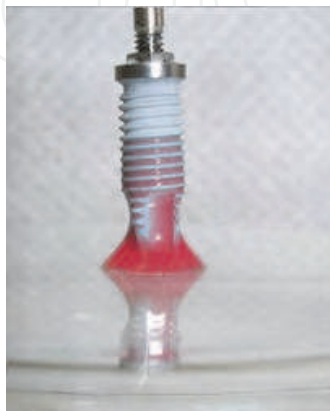
Fig. 4. Vulcano Actives™ dental implant showing its high hydrophilic surface.
