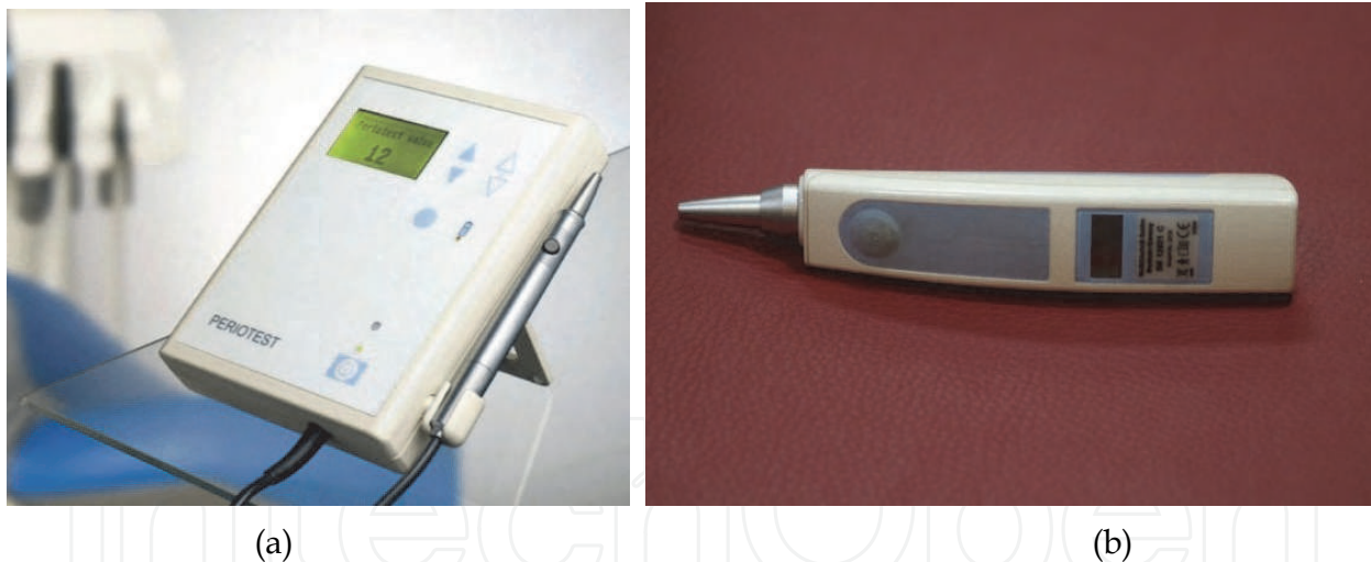
Fig. 2. Periotest ® (Siemens AG, Bensheim, Germany) measures tooth mobility and implant stability by periotest value (PTV). (a) Periotest ® , (b) Periotest ® M.
