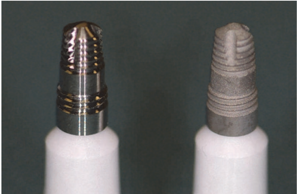
Fig. 3. The machined and nano etched implant surface
