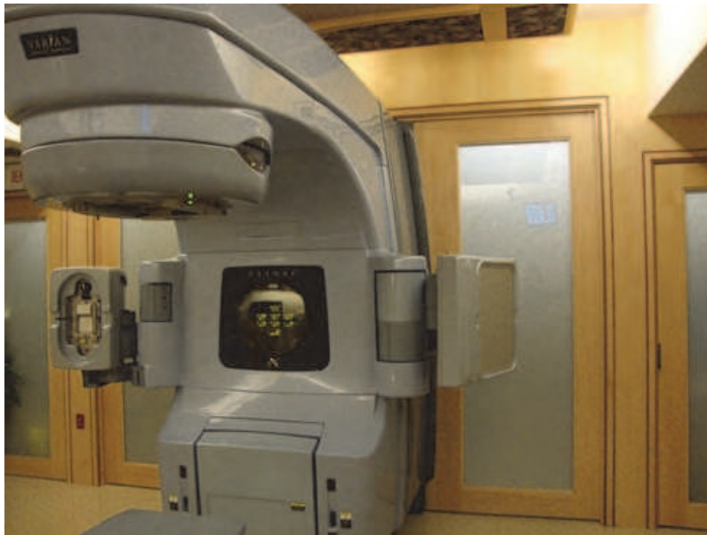
Fig. 10. Linear Accelerator with kV imaging arms attached. VARIAN 23 iX with OBI (On Board Imager).
