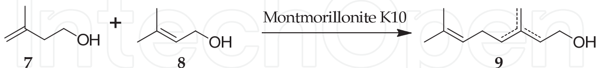
Scheme 7. Biomimetic condensation of isopentenol 7 with prenol 8 induced by montmorillonite K10.
