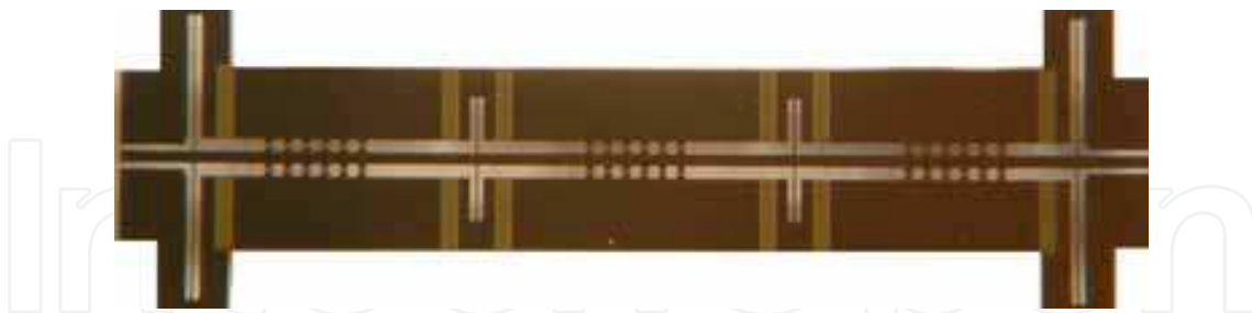
Fig. 21. A prototype of a 3-pole SWR filter with a total of 8 DC blocking capacitors
