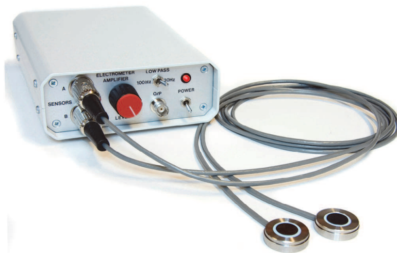
Fig. 3. Photograph of one embodiment of the EPS electrophysiology system, comprising a pair of insulating electrodes and a differential amplifier with analogue output.
