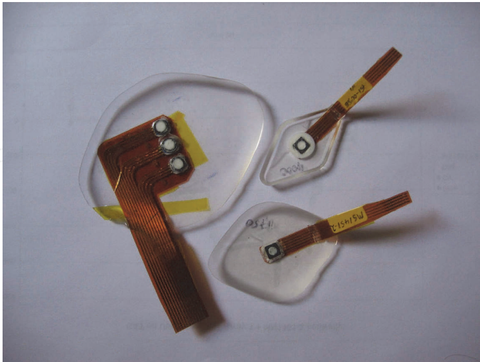
Fig. 4. Discrete and array Biomedical Interface Pressure Transducers (BIPT) incorporating modified MEMS pressure sensors.
