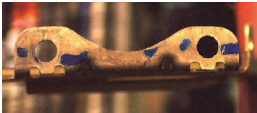
Fig. 8. Sample fail (missing clip) for the orientation image set.
