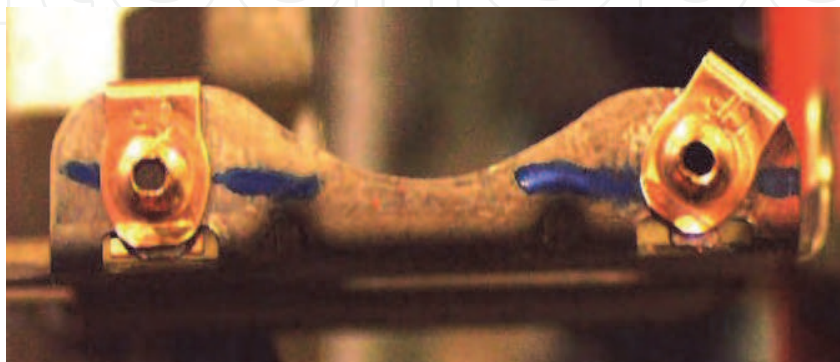
Fig. 9. Sample fail (backwards and upside down clip) for the orientation image set.
