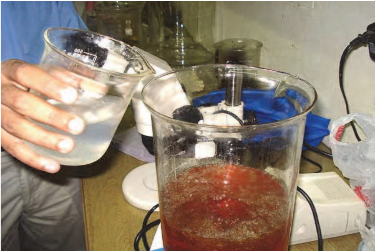
Plate 3. Mixing of sodium methoxide catalyst
