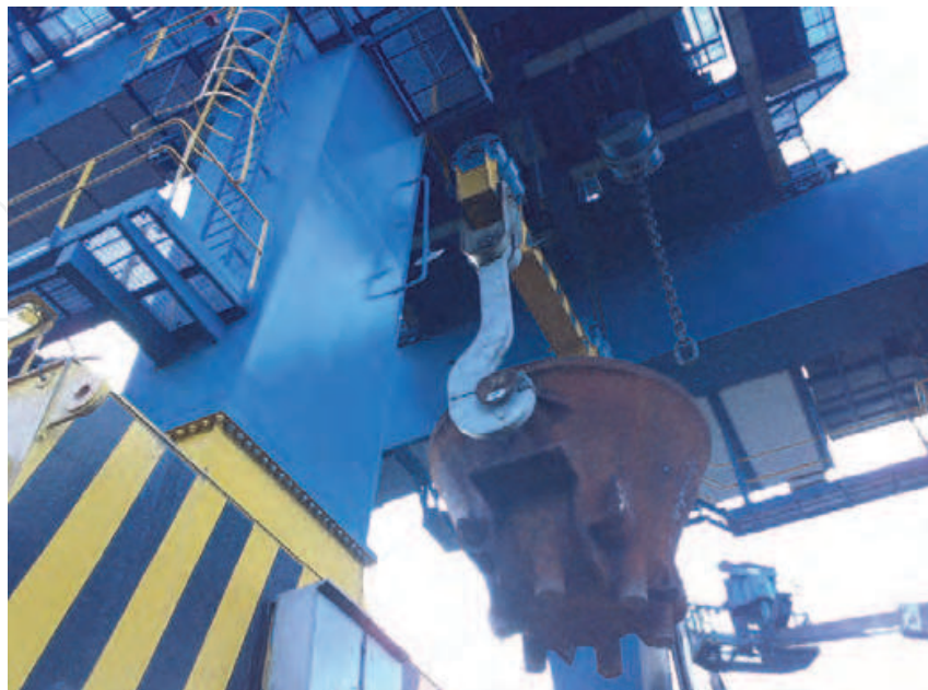
Fig. 14. Slag vessel on the transport crane.
